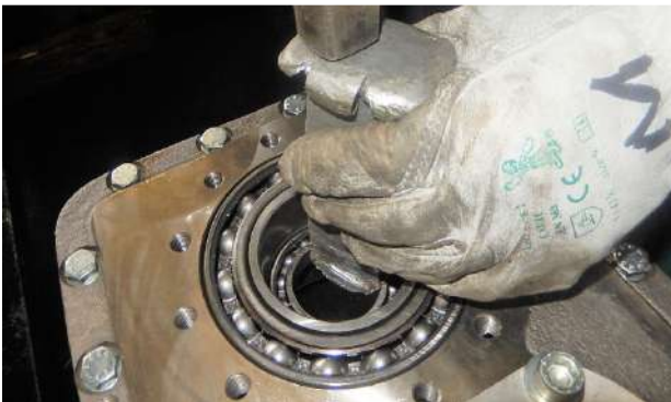
Put the assembled case with the cover into the upper part. Insert the bearing 6010 #84 into the gear ( z=25 ).
