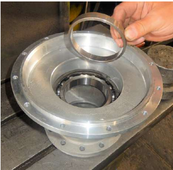
Insert the spacer #27.
