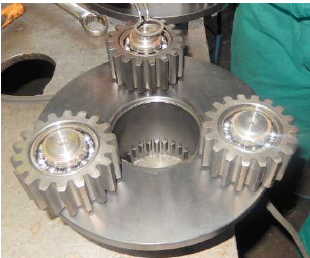
By a means of a proper pliers put the elastic ring E25 #26 in the proper seat.
