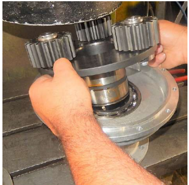
Plant the second bearing 6019.
