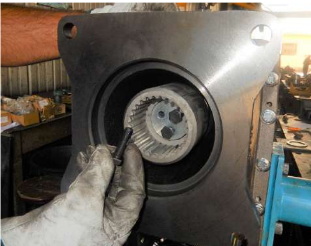
Insert the elastic ring #89.
