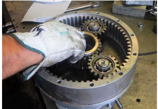
Position the shim on the solar gear.
