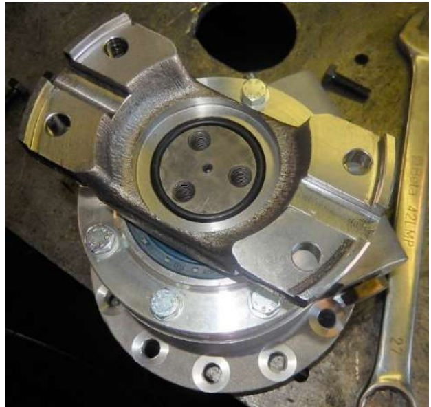
Insert the fork C6 #58 on the shaft. Position the OR ring.
