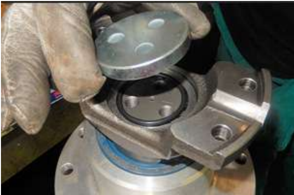
Insert the OR ring under the three holes washer
