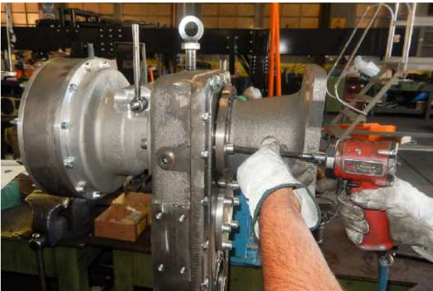
Install the motor support on the case (screws 12x1,75x35 + conic washers) (allen key 8 mm)
