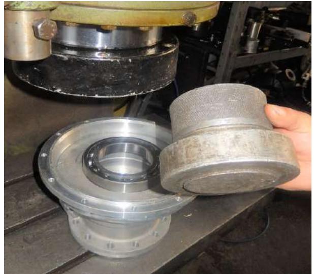
Put the case under a press and position the first bearing 6019 #7.
