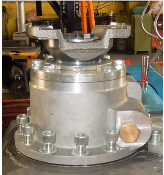
Install the rear axle disconnection group on the case. (Tighten the screws 12x1,75x35 + conic washer, allen key 8 mm)
