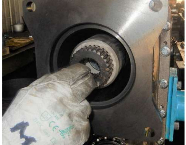
Insert the intern entrainment sleeve #88.
