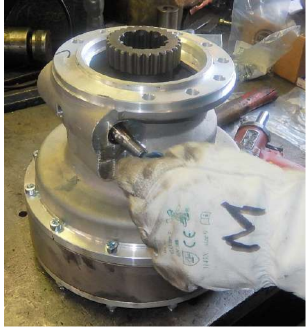
Insert the oil seal # 71 on the fork shaft.
