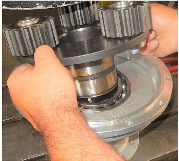
Extract the planetary holder.
