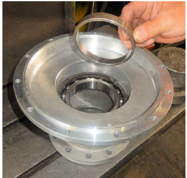
Remove the plastic ring of the bearing and the bearing from the case.
