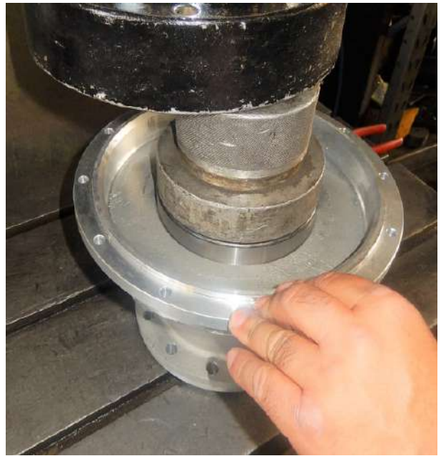
Plant the second bearing 6019.
