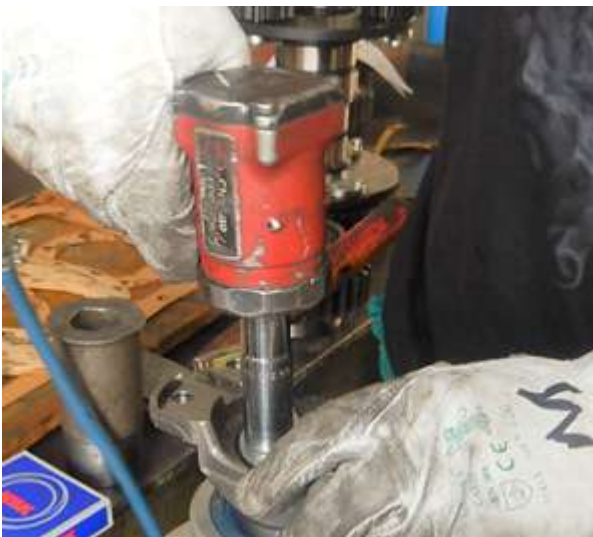
Tighten the screws 10x1,5x35 10.9 (socket wrench 16 mm).
