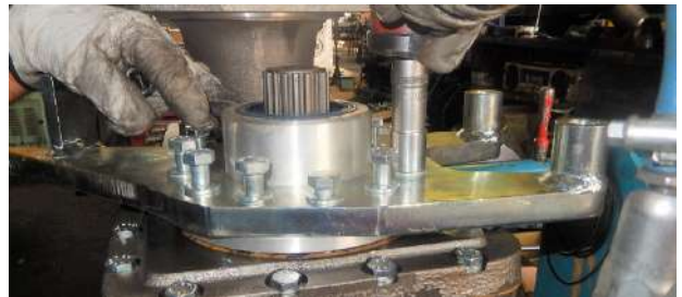
Mount the brake cylinder support #60 (screws 12x1,75x55 with wave washer, socket wrench 18 mm).
