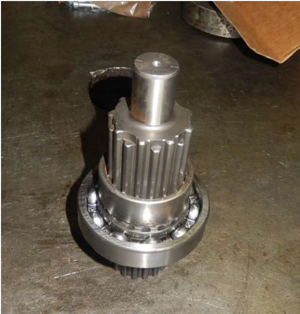
Insert the spacer ring #82
