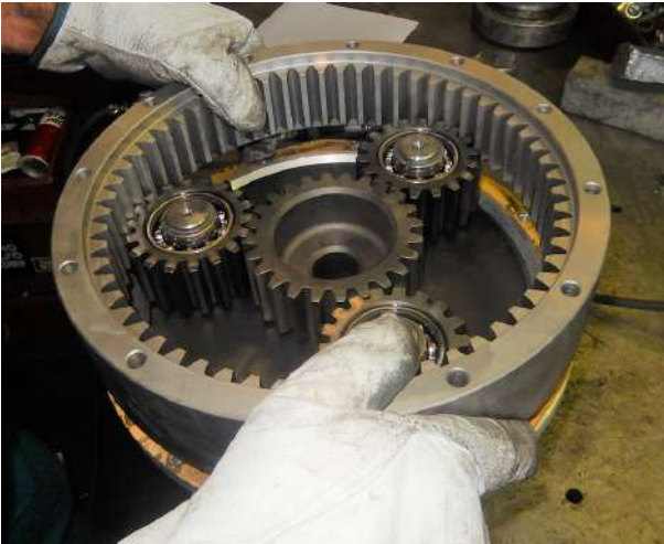
Insert the internal toothed wheel #43 on the satellites.
