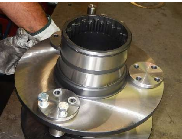
Remove the pins (for screws Ø8 use a socket wrench 13 mm).
