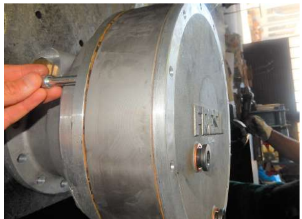
Inset the allen screws 10x1,5x100 for fixing.
