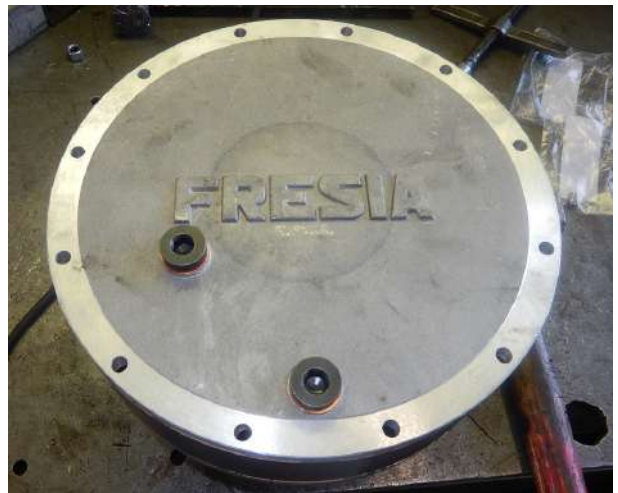
Screw the cover on the group and install the oil plugs with copper washers.
