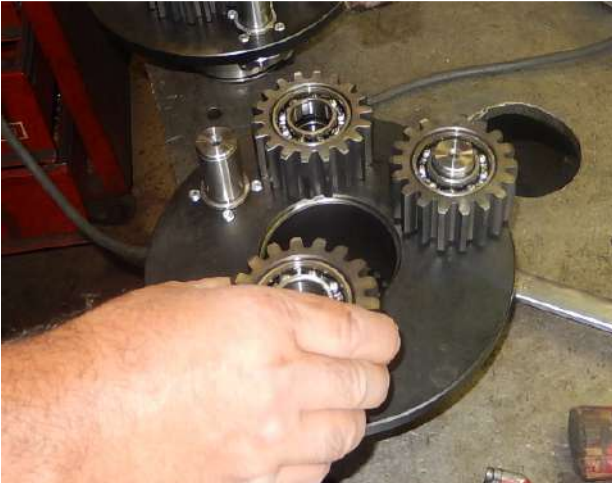
Heat the bearings with a thermic gun to extract them easily.
