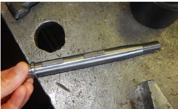
Insert the splines into the fork shaft.
