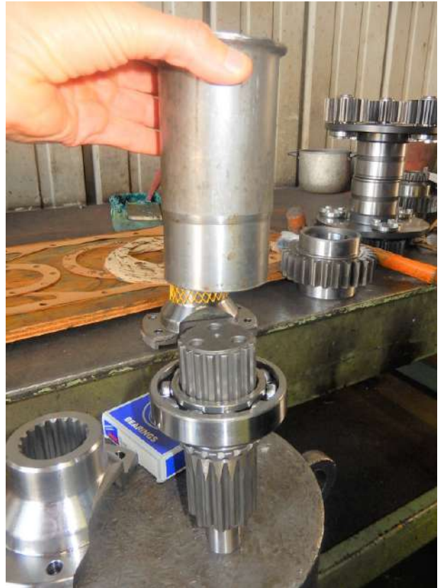
Plant the bearing 6210 #44 on front output shaft.
