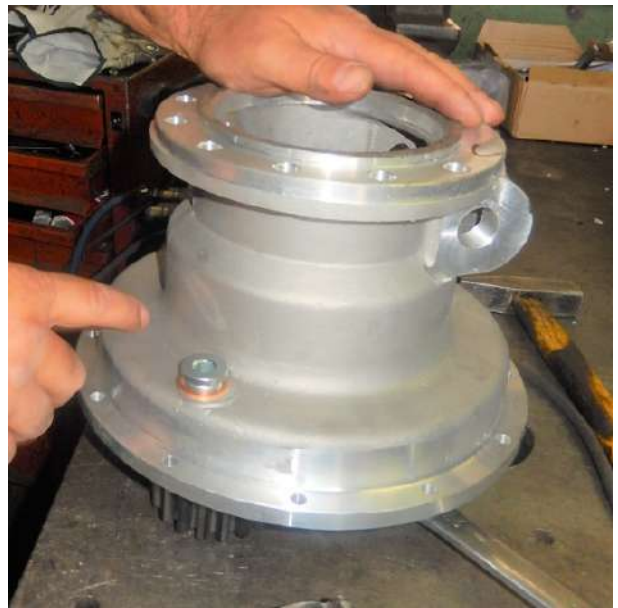
Put the plug #69-70 and copper washer.
