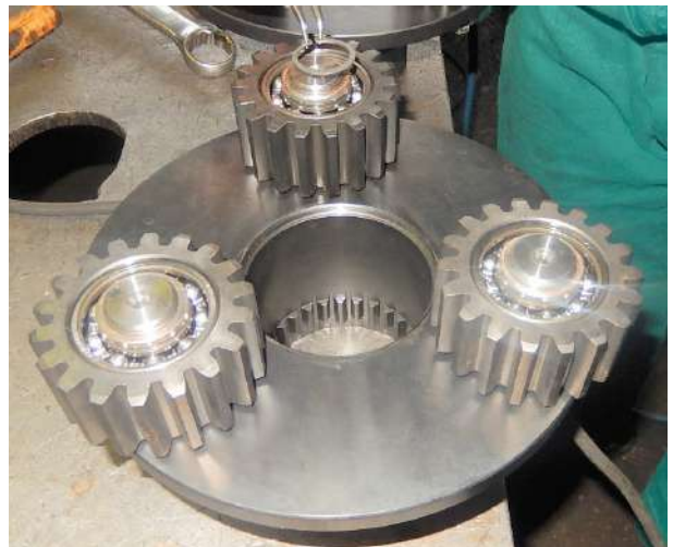
By a means of a plier, remove the elastic rings fixing the satellites to the pins.
