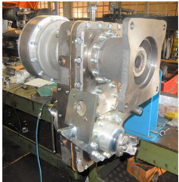
Put the oil plugs with copper washers on the transfer. (PICTURE OF THE TRANSFER ASSEMBLY)
