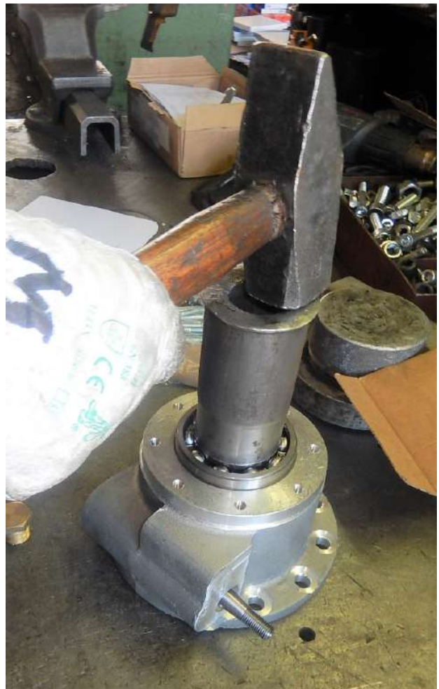
Beat slightly on the bearing by a proper punch plant the shaft and the bearing.
