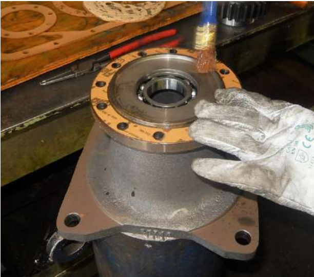
Rotate the support and position the paper gasket (lubricate it)
