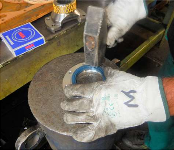
Insert the oil seal 70x90x10 #59 into the cover. Be careful not to damage it.
