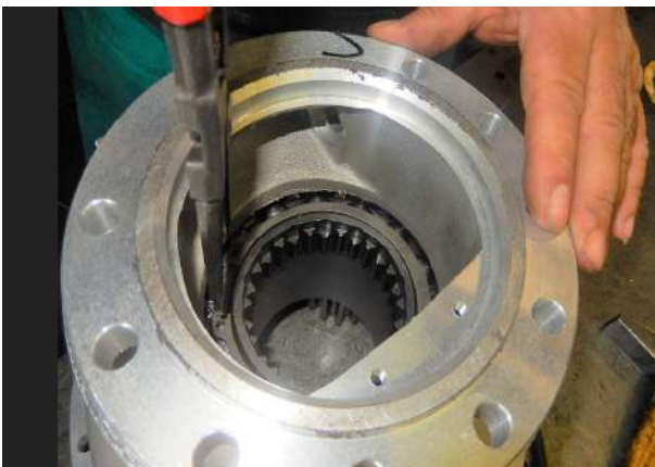
Rotate the group and insert the elastic ring E95 for fixing. (use the proper pliers).
