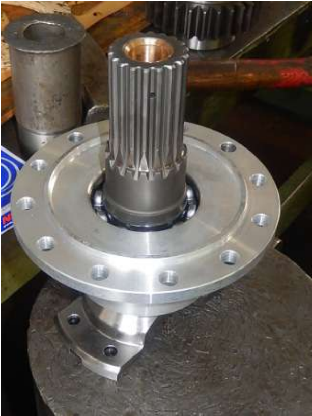
Plant the bronze bushing #66 on the shaft.
