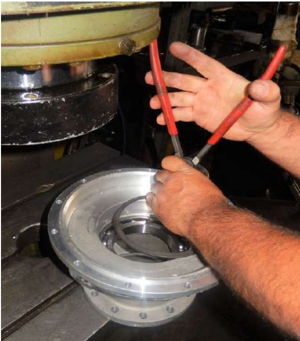
By the pliers, insert the elastic ring I145 #18 to fix the bearing.
