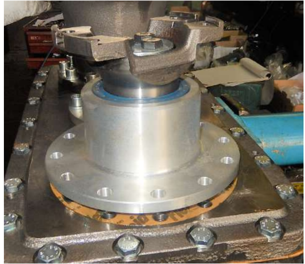
Put the assembly of the output shaft on the case. Lubricate the paper gasket and put it between.
