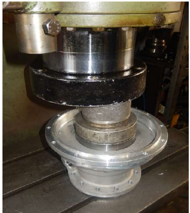
By a means of the proper beater, insert the bearing in the bottom of the case.
