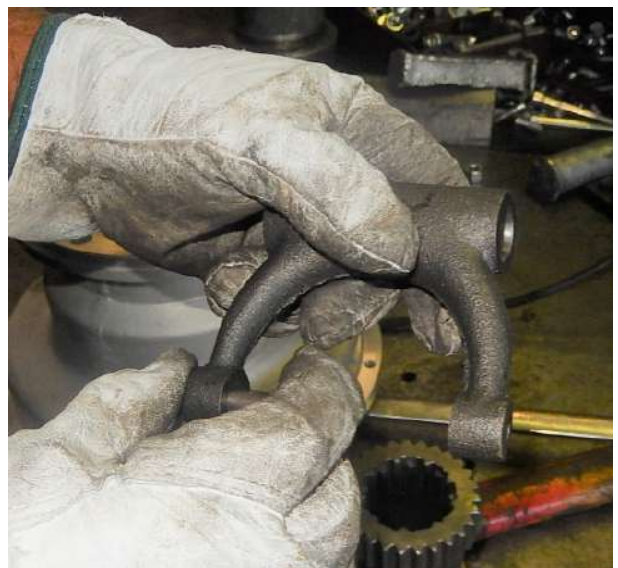
Put the sliding element #37 in the fork.
