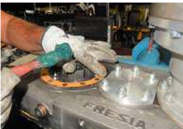
Rotate the case and insert the paper gasket, before lubricate it.
