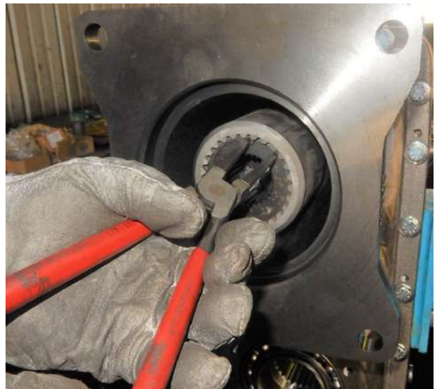
Insert the elastic ring #89.
