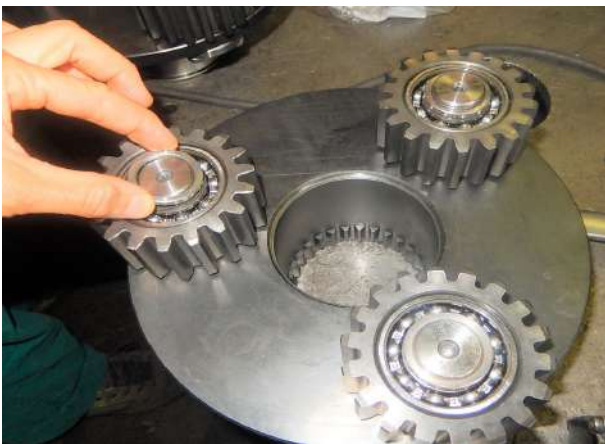
Put the shim on the opposite side.
