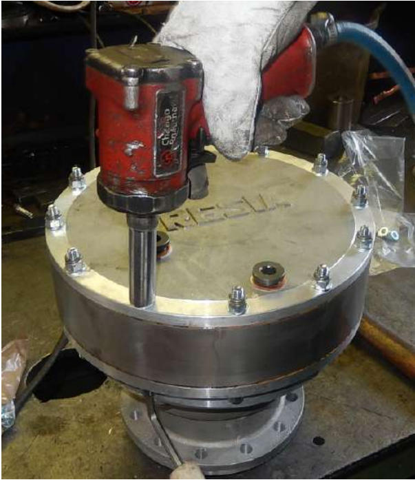
Tighten the nuts on plane washers.
