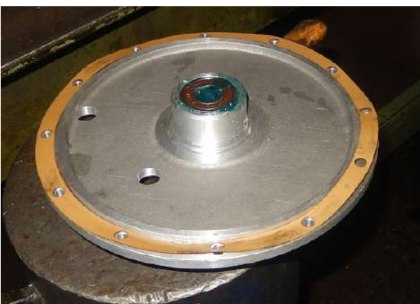
Put the paper gasket #41 on the edge.
