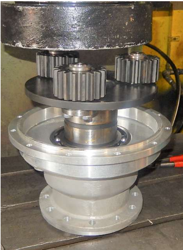
Insert the planetary group into the case by a means of the press.
