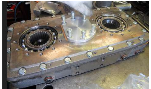
By a means of proper pliers, extract the elastic ring I90 #45.
