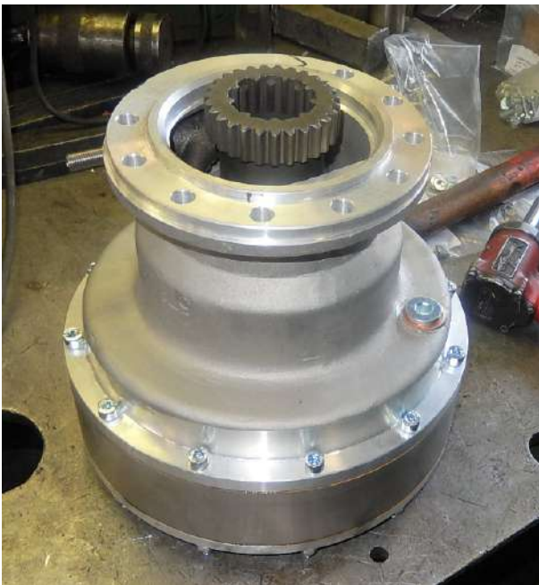
Rotate the planetary group and insert the toothed sleeve #39 into the sliding elements of the fork.
