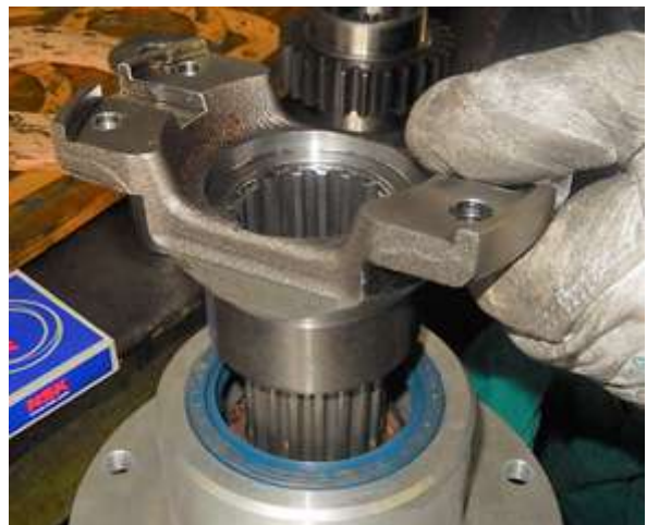
Insert the fork on the output shaft C6.
