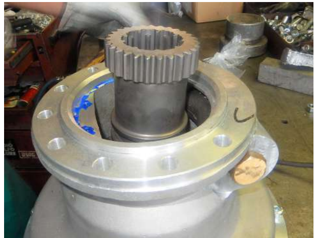
Spread the Loctite MEDIUM on the oil protection carter seat .
